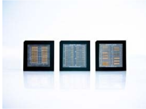
Individual emitters or emitter bars by lithography process
